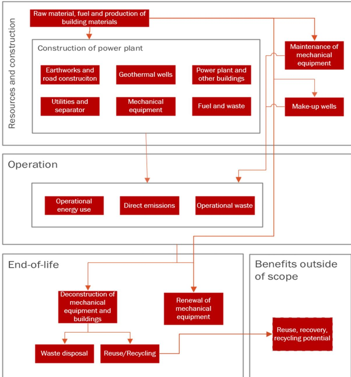
**Figure 2.1** The main unit processes set up to describe the production of electricity and heat from Reykjanes power plant.
