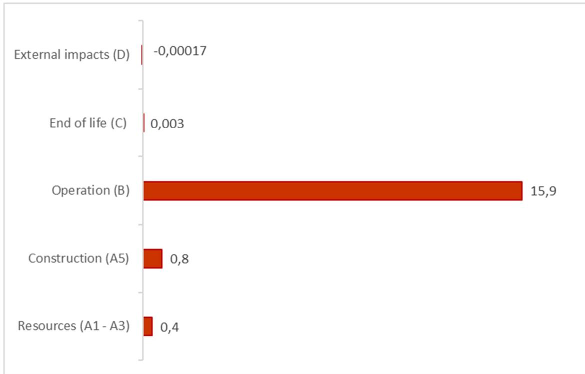
**Figure 4.2** Carbon footprint for each life cycle stage of Reykjanes power plant.
